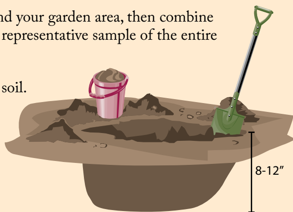
Slice for sample: 8-12 inches long by 1-1½ inches thick.
